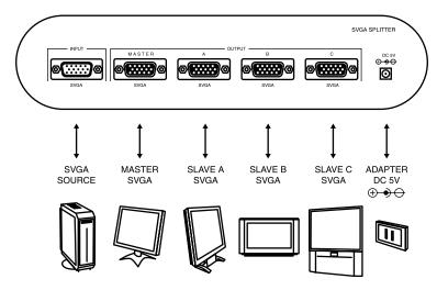
1. Connect the SVGA cable between the SVGA source and B114-0H4 splitter marked 'INPUT'.
